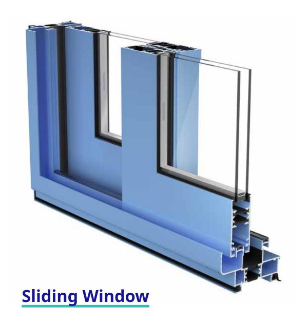
This generic double slider has a frame thickness of 93 mm and a sash of 29 mm, with a possible glazing up to 38 mm.
